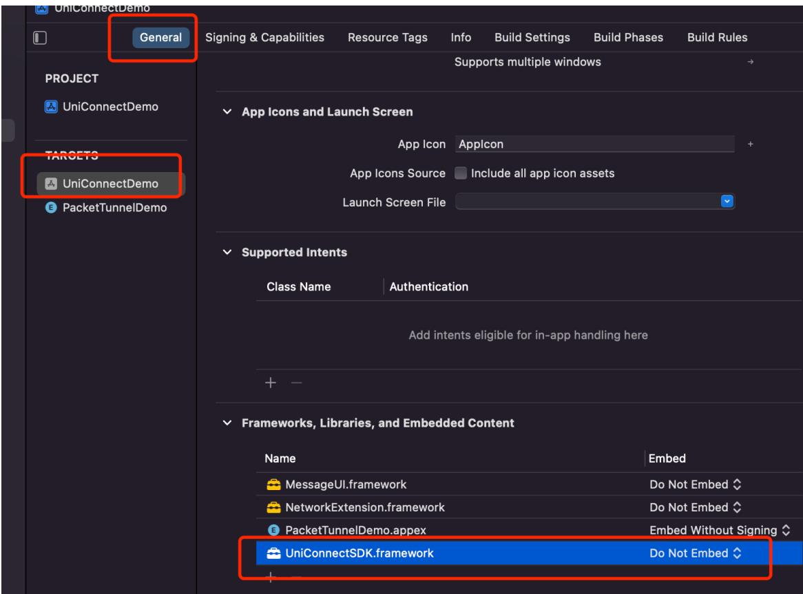
The screenshot shows the Xcode General settings for the UniConnectDemo target. The 'General' tab is selected. In the 'Frameworks, Libraries, and Embedded Content' section, the 'UniConnectSDK.framework' entry is highlighted with a red box, and its 'Embed' dropdown is also highlighted with a red box and set to 'Do Not Embed'.
